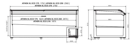
\* Universal cabinet: The cabinet covers all three temperature ranges of refrigeration +3 °C to +15 °C / meat and minced meat refrigeration 0 °C to +2 °C / freezing –18 °C to –23 °C.
